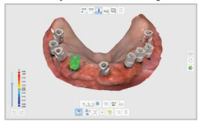
Abutments and scan bodies are automatically matched and aligned with the scan data. Use this function for downstream work such as CAD.
